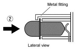
3. Rotate a xenon bulb pushing it and adjust notch to a metal fitting.
